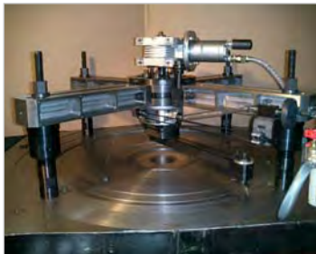
XP1200 Planen / Facing: 0 mm – 1200 mm Spannen / Clamping: 500 mm – 1400 mm
