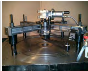
XP1800 Planen / Facing: 300 mm – 2800 mm Spannen / Clamping: 500 mm – 2050 mm
