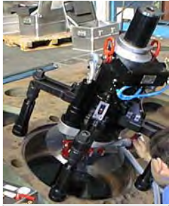
TA240 Planen / Facing: 0 mm – 1000 mm Axial Hub / Axial Stroke: 240 mm
