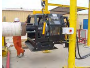
High Speed Beveler US80/150 HSB 168,3 mm – 355,6 mm US220 HSB 323,9 mm – 558,0 mm US420 HSB 558,0 mm – 762,0 mm US620 HSB 762,0 mm – 965,0 mm US820 HSB 965,0 mm – 1220,0 mm
