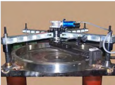
XP2000 Planen / Facing: 685 mm – 2010 mm Spannen / Clamping: 750 mm – 2300 mm
