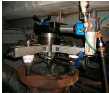
MS600 Planen / Facing: 0 mm – 600 mm 2 driving motors: 2x 750 W
